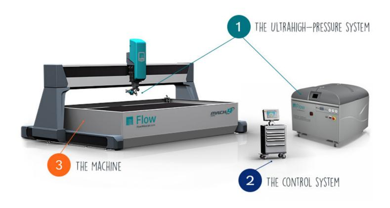
With the shapecutting machine tool, the material is placed (or fixtured) on a work table and the cutting head is moved in an XY plane over the top. Sometimes the head has five axes of motion for bevel or 3D cutting.
